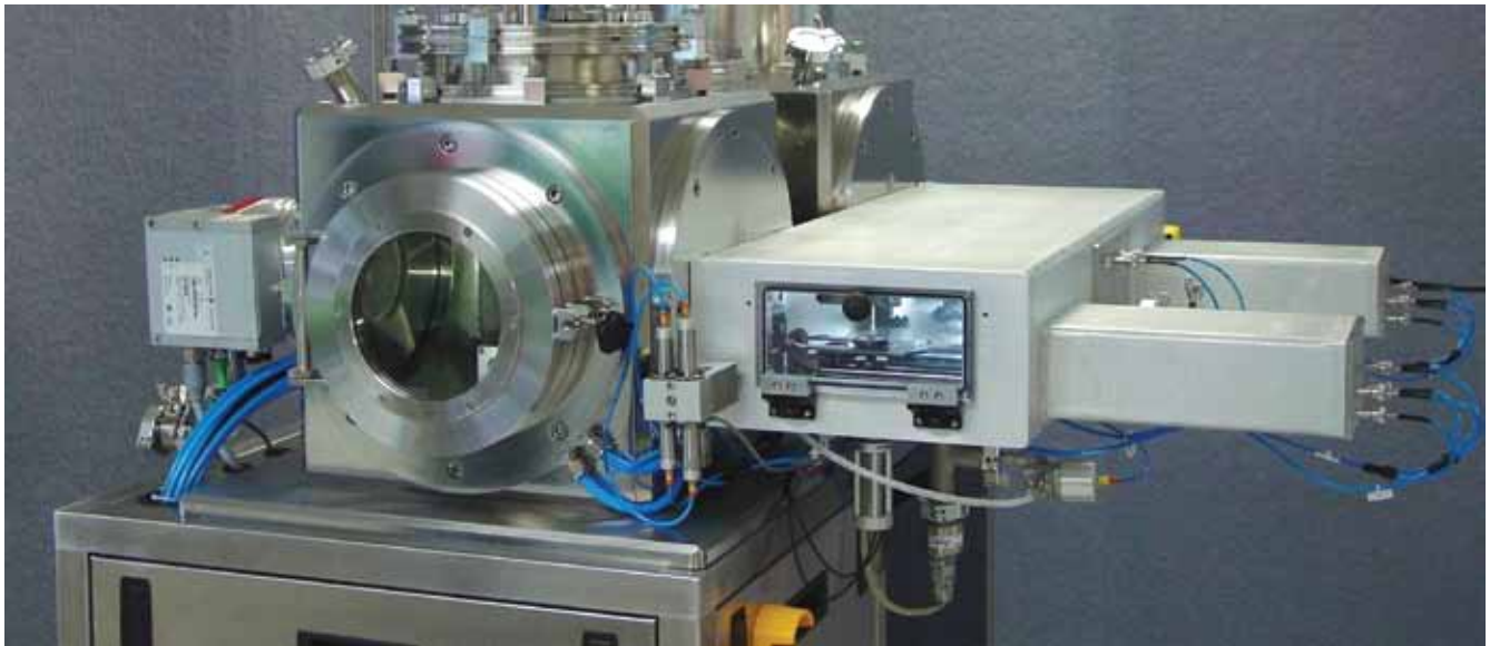
Dual Chamber Ion Beam Milling/Etching and Sputter Coating in Vacuum Sample Transfer
